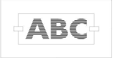
Tape the decal in the proper location with 1"-2" strips of masking tape placed across the middle of each side of the decal, as shown above. Make sure the decal is positioned exactly where you want it. Measuring to a reference point is recommended.
